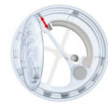
When the membrane is unrolled, it locks to a magnet in the housing, thus keeping the valve closed for speech.
