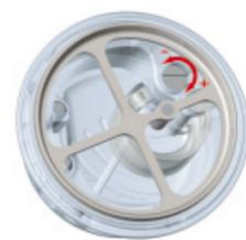
Turning the screw alters the magnet distance and thus the force needed for opening.
